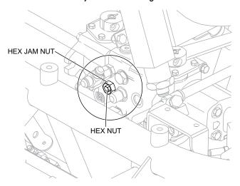
Figure 49. Steering Pressure Adjustmen
